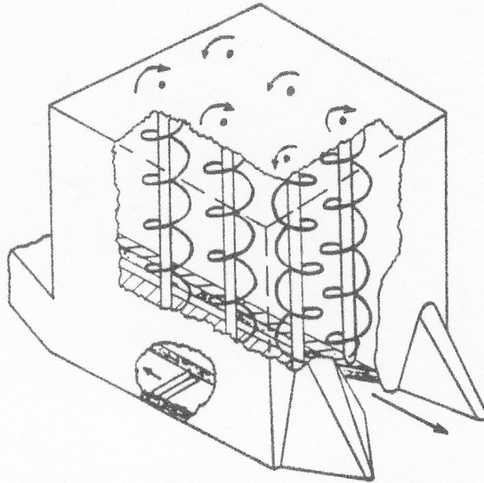
Figure 3. Vertically-oriented, twin, single open-helix chile harvester manufactured by Wondel Creager, Salem, New Mexico, U.S. (Creager 1971).
