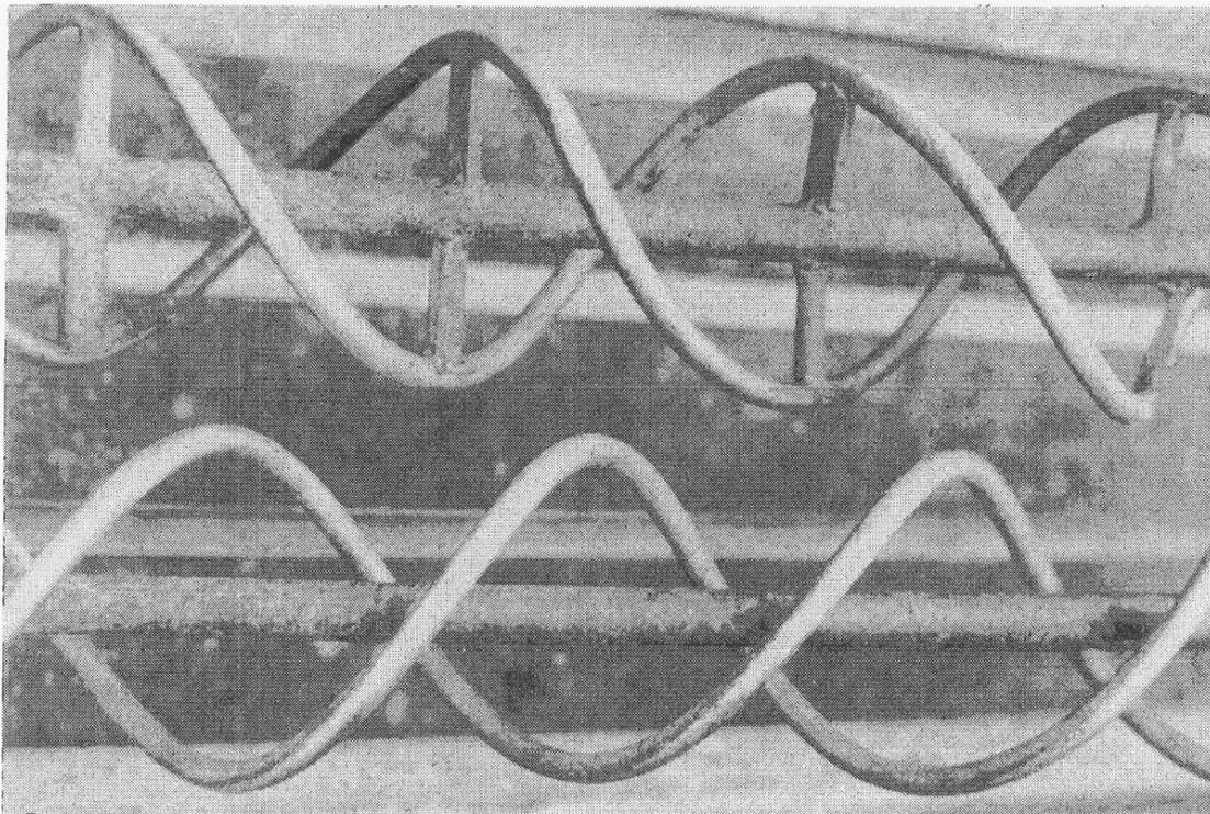
Figure 5. Experimental, twin, double open-helix concept (160 mm diameter shown) tested on pimienta peppers in Georgia, U.S. (Fullilove and Futral, 1972)
