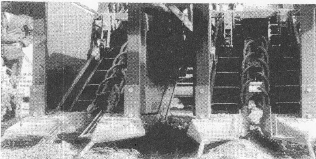
Figure 6. Experimental two-row, 160 mm diameter twin, double open helix self-propelled harvester for chiles for dehydration; built by the Agricultural Engineering Institute, Israel (Wolf and Alper, 1985).
