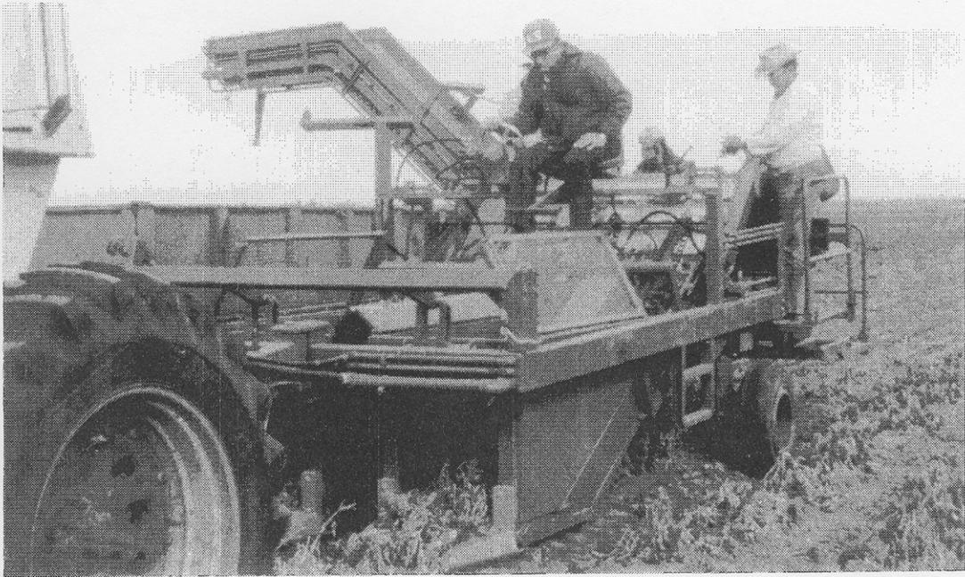
Figure 7. Commercial two-row, twin, double open helix trailer harvester for chiles for dehydration tested in Texas; manufactured by Sharnoa, Ltd., Israel.
