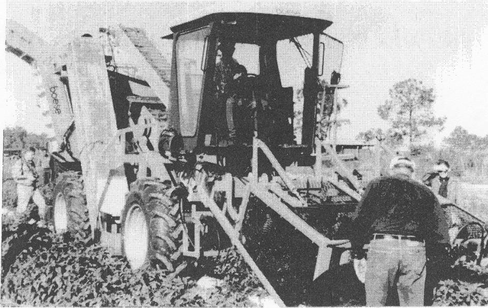
Figure 9. Commercial two-row, twin, double open-helix, self-propelled, pepper harvester manufactured by Boese Equipment, Saginaw, MI, U.S.
