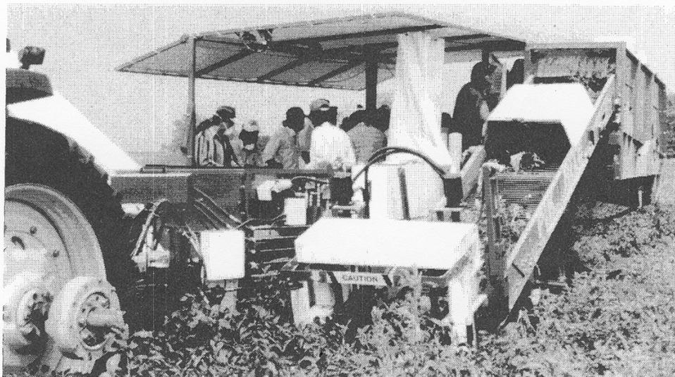
Figure 10. Commercial, powered, oscillating, forced balance shaker with soft-coated fingers, trailer pepper harvester, originally developed for harvesting tomatoes; manufactured by Pik Rite, Lewisburg, Pennsylvania, U.S.
