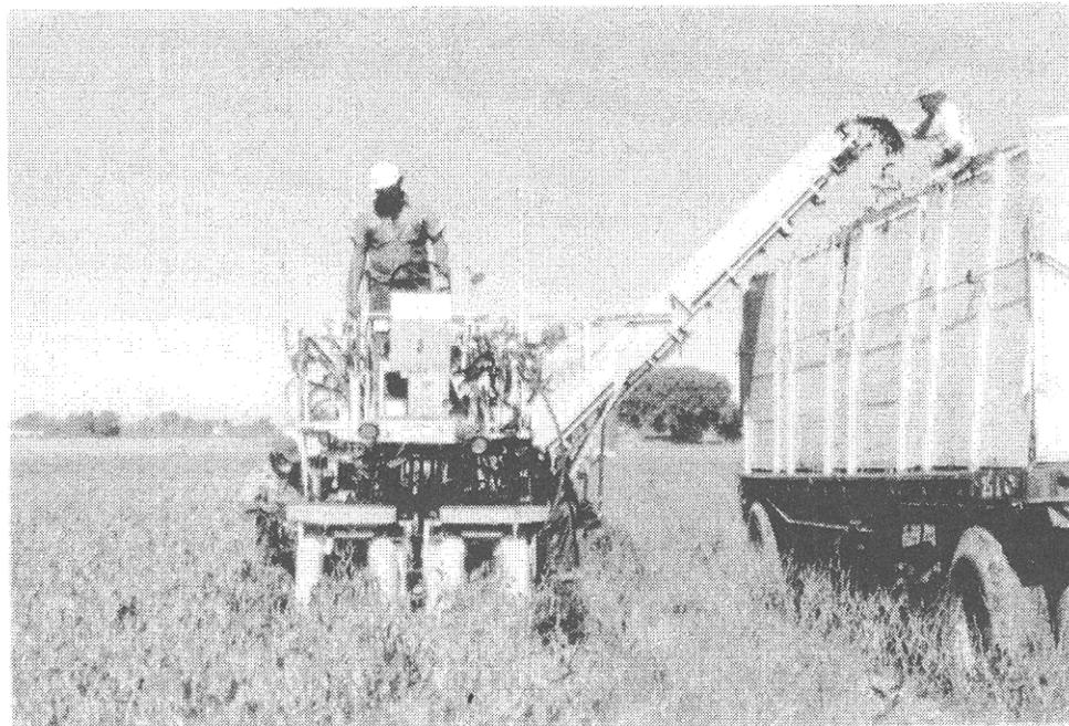
Figure 2. Inclined, counter-rotating brush chile harvester built by Cal Compack, based on Riggs' 1971 patent.
