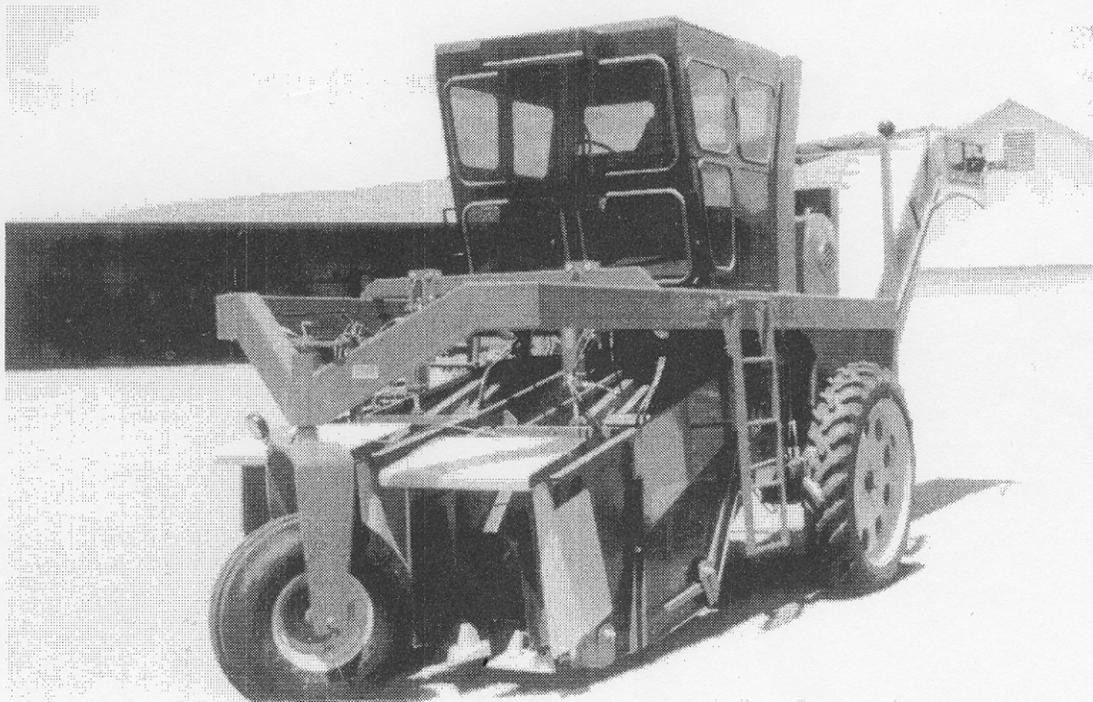
Figure 8. Commercial two-row, twin, double open-helix self-propelled, pepper harvester manufactured by McClendon Welding, Tulia, Texas, U.S..
